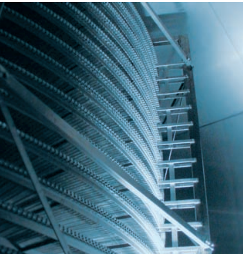
Low floor space requirement by using the room height: MIWE spiral freezer.
