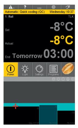
The main display of the MIWE TC: Efficient and with a clear layout, it displays all parameters in graphic or alphanumeric form. The black blocks stand for the individual phases with the respective setpoint setting; the yellow graph shows how the MIWE TLK converts the setpoint values into actual temperatures in real time, whereas the blue graph shows the humidity.
