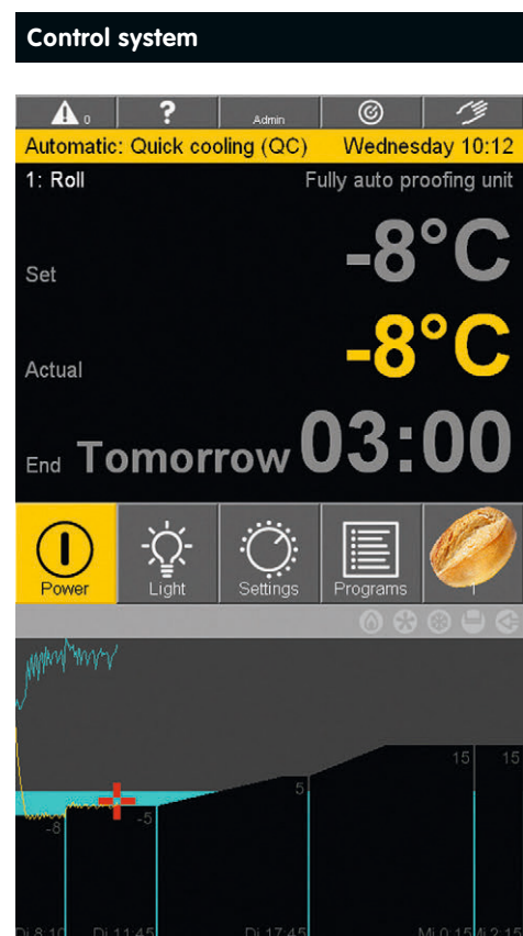
The main display: Efficient and with a clear layout, it displays all parameters in graphic and/or alphanumeric form. The black blocks stand for the individual phases with the respective setpoint setting; the yellow graph shows how the MIWE GVA converts the setpoint values into actual temperatures in real time, whereas the blue graph shows the humidity. You will find other screen shots on the last page of this product information.
